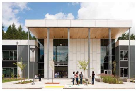
Key sustainability features include orientation and extensive use of skylights for daylight harvesting, rainwater capture system for toilet flushing, pervious paving and bioswales for storm water management, infrastructure for photovoltaic system, high-efficiency air-to-water heat pump and modular construction, which leads to less material waste and lower embodied energy.
